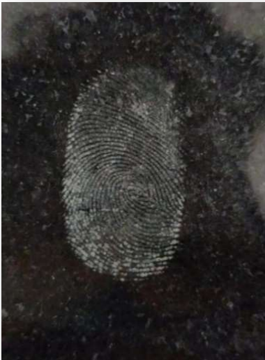
Figure 4: Development of Latent Fingerprint with the help of Banana powder on a porous marble surface
