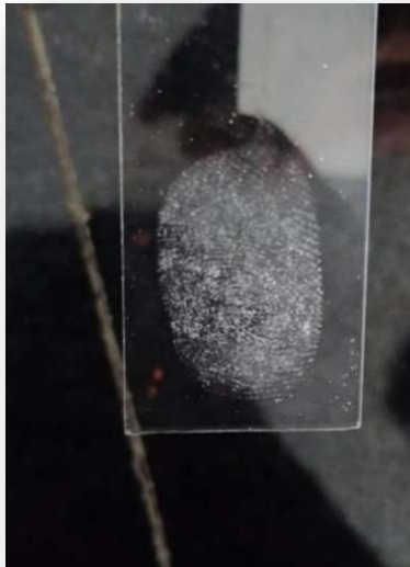
Figure 5: Development of Latent Fingerprint with the help of Neem powder on a porous marble surface.
